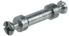
System 2 piece Double H.263.24.943 *2 Piece bolt for Fixed Shelves. Cam system Locks onto this Bolt Place on middle Gables/Panels that have another fixed shelf on the other side
