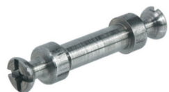
System 2 piece Double H.263.24.943 *2 Piece bolt for Fixed Shelves. Cam system Locks onto this Bolt Place on middle Gables/Panels that have another fixed shelf on the other side
